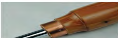
This copper ferrule has developed a warm patina over time. I often select a ferrule that will complement the wood.
