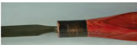
Three separate pieces of ebonized copper pipe butted together make a utilitarian ferrule. With use, the black wears off and the ferrule develops a fine patina with the copper showing through.
