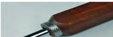
I cut this ferrule from a textured bathroom towel bar.
