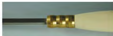
This ferrule is made from three brass natural-gas fittings.
