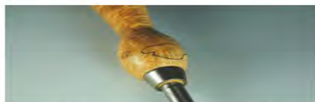
A spacer-lug from a truck tire becomes a sturdy ferrule.
