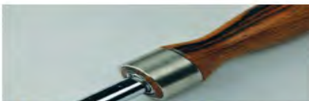
This stainless steel ferrule came from pipe that I salvaged from a boat. Stainless steel is hard to cut but it is strong and looks good with any wood.
