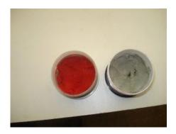
Take equal amounts of Part A and Part B and mix them together – Have a small dish of water handy to make the process smoother – after mixing – Place the Apoxie Sculpt in the flute and be sure and push it to the bottom of the flute – Need some overlap of the Apoxie Sculpt – After filling all the flutes, it will require at least 24 hours to completely set and harden.
