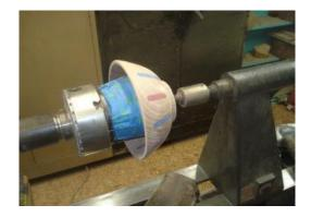
Finish – I finish with Deft Lacquer (Satin) – Apply lacquer – rub with steel wool – spray lacquer – rub with steel wool – etc – I will continue this process until I am satisfied with the finish and the look of the piece.
